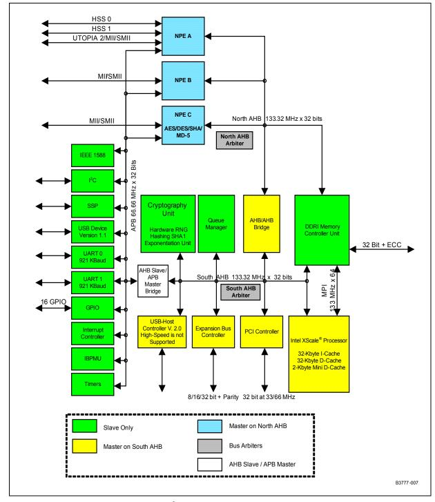
*Note:* Figure 1 shows the Intel<sup>®</sup> IXP465 Network Processor. For details on feature support listed by processor, see the *Intel<sup>®</sup> IXP45X and Intel<sup>®</sup> IXP46X Product Line of Network Processors Datasheet*.
